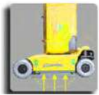
Automatic Pothole Protection
